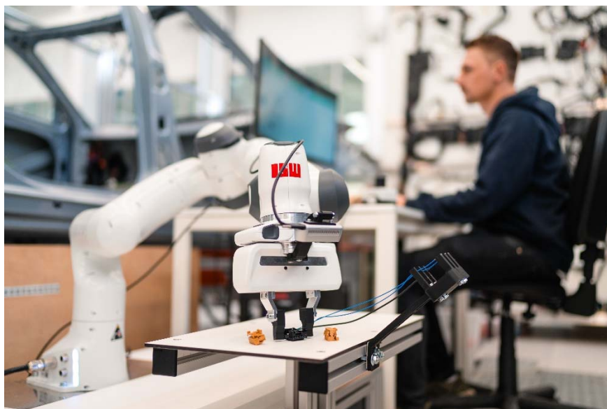
The robot uses optical sensors to detect the position of the connectors and automatically installs them with cables. © Ludmilla Parsyak, University of Stuttgart
