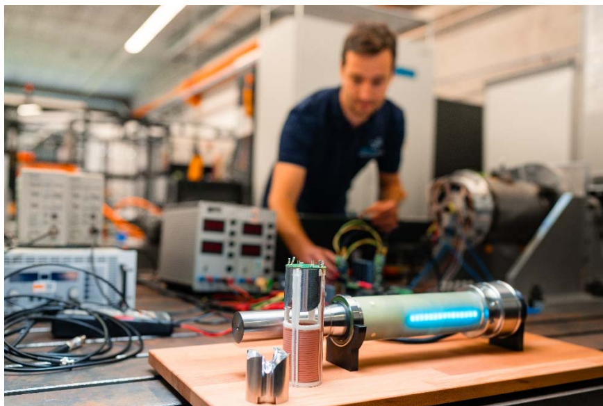
Hybrid rotor shaft made of glass-fibre-reinforced plastic and steel for the inductive electric excited synchronous machine. © Ludmilla Parsyak, University of Stuttgart
